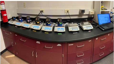
Image Caption: Figure 1. HYPROP collecting data for soil water retention curve.
