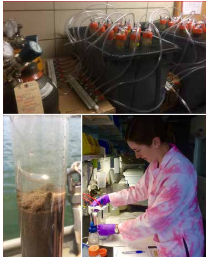
Figure 2. Sediment core incubation system (top), cores collected from study lakes (bottom left), and analyzing water samples for phosphorus (bottom right).
