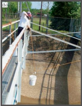
Figure 3: (a) High-resolution sampling of soil pit in an upland field. (b) Collection of a suspended sediment sample from a bridge.
